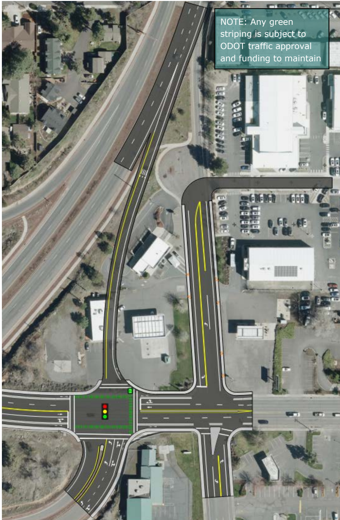
FIGURE 11. ALTERNATIVE 2 AT REED MARKET ROAD/US 97 NORTHBOUND RAMP
